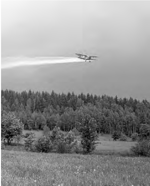
Spraying was primarily carried out by AN-2 biplanes, known as 'budgerigars' (photo Jan Vaněk)
